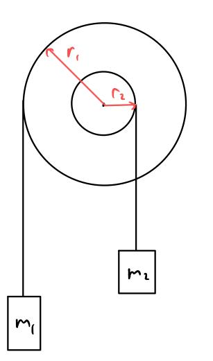
$r_1 = 50 \text{ cm}$   $r_2 = 20 \text{ cm}$   $m_1 = 1 \text{ lg}$  $m_2 = 2 \text{ lg}$
