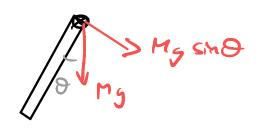
(whit was T, ?  $T, = T_{cn} + M(\frac{L}{2})^{2}$  parallel axis then 8 from take,  $T_{cn} = \frac{1}{12} M L^{2}$   $\Rightarrow T_{c} = \frac{1}{12} M L^{2} + \frac{1}{4} M L^{2}$   $= \frac{4}{12} M L^{2} = \frac{1}{3} M L^{2}$ So
